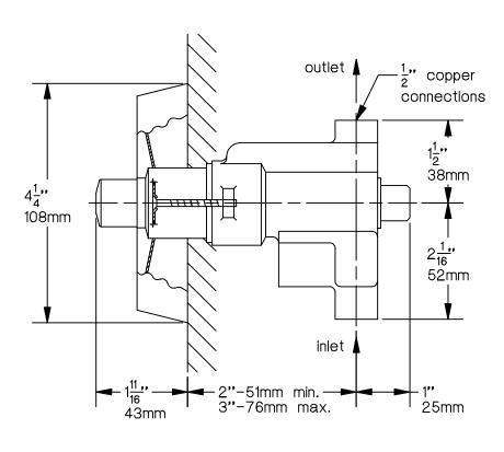
illustrated 3"-76mm from centerline of tubing to face of wall.
